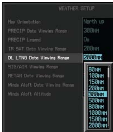
Figure 4-112 GFDS Lightning Viewing Range Selection
